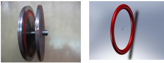
Figure 3. -Matrix for the execution of silicone gasket
